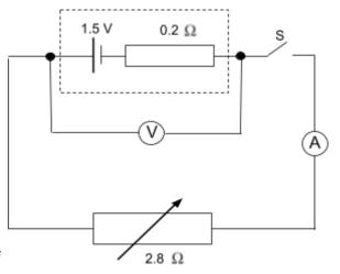
4) A physics student set up the following circuit to investigate an electric cell.
