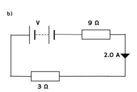
4) Find the potential difference across each resistor in the circuit below.
