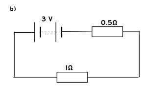
3) In the circuits below find the value, V, of the dc source's voltage.
