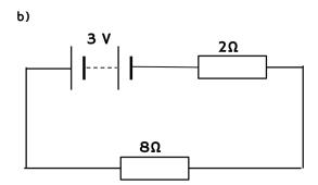
2) Show that the potential differences (pds) across each resistor in the circuits below adds up to the source voltage of the circuit.
