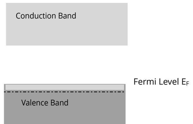
A p-type semiconductor is made by adding an element from group 3 to the silicon crystal. This creates holes in the valence band.
