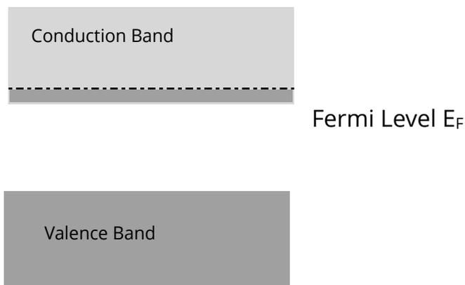
An n-type semiconductor is made by adding an extra electron by doping the semiconductor crystal with an element in group 5.
