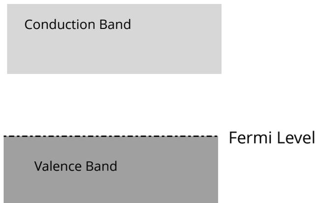
For a pure semiconductor the valence band is full and the conduction band is empty.
