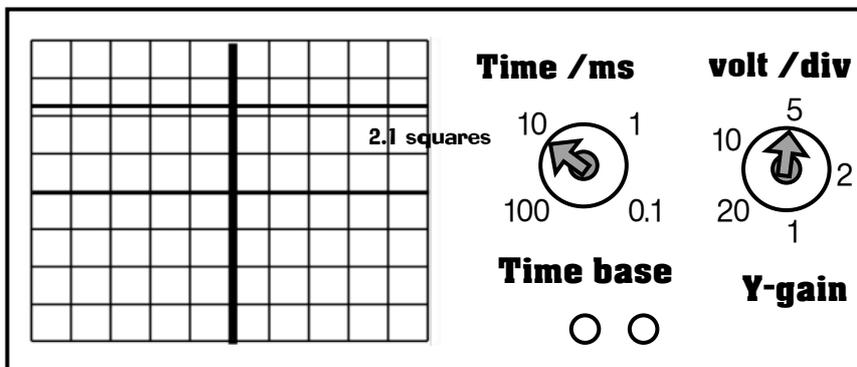
Direct current voltage from the dc source connected to the lamp giving the exactly **same brightness.**
