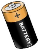
The electric current produced by a cell flows in one direction around a circuit. The chemical reaction in the cell makes an emf which acts in one direction. This kind of electricity is called **direct current** electricity or d.c. For short.
