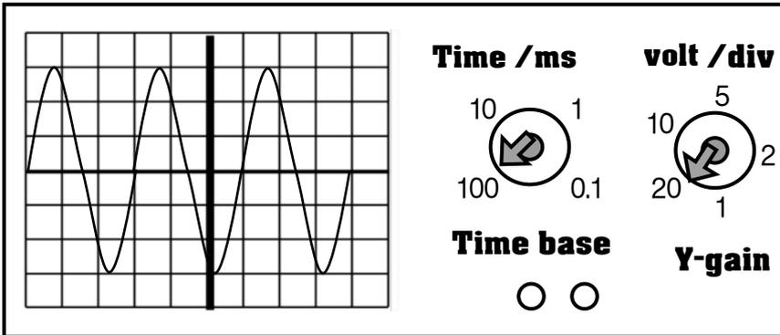
Find the peak voltage and the root mean squared voltage from the a.c. signal.
