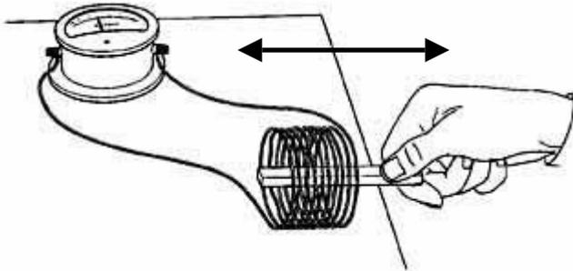
Electric current can be produced with a magnet and a coil of wire.
