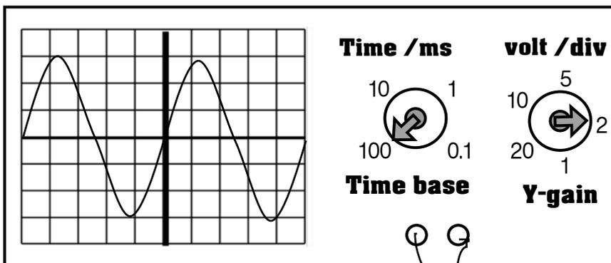
Attaching the coil to an oscilloscope shows the variation in the produced emf and the current.
