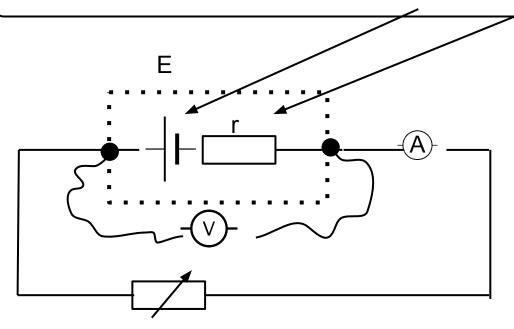
When no current is taken from the cell the voltmeter across the terminals measures the EMF of the cell.
