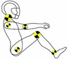
Car safety has vastly improved with the help of sophisticated dummies fitted out with accelerometer and force sensors.
